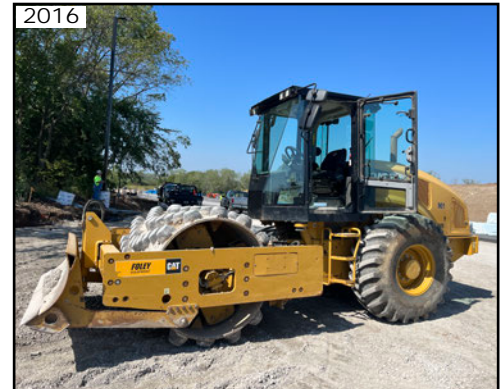
2016 Caterpillar CP56 Compactor w/Blade
