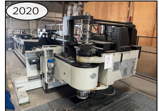
2020 BLM Model Elect-XL Hydraulic Tube Bender, 12-Axis, 6" Max Tube Bending Capacity - Huge Qty. of Tooling
