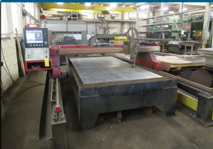
Lincoln Pro Line 2200 Precision Plasma Cutting System w/Lincoln Electric Burny 10LCD Control
