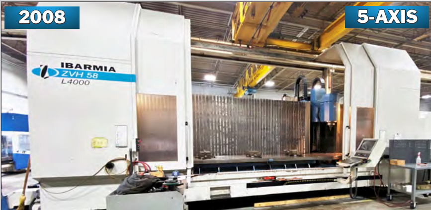
2008 5-AXIS IBARMIA ZVH 58 L4000 5-AXIS CNC TRAVELLING COLUMN VERTICAL MACHINING CENTER
