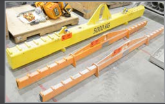
MLE SERVICES spreader beams
