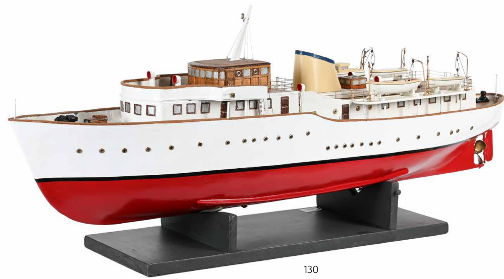
130 A FINE MODEL OF A LIVE STEAM YACHT BELIEVED TO HAVE BEEN BUILT IN THE 1950s - 1960s With detailing to include wheel house, gallery rails, lamps, vents, anchor, planked decking twin masks with rigging, lifeboats and large funnel. The model constructed from solid wood planking and framing. The horizontal gas fired steam plant driving a live steam engine with horizontal copper boiler having pressure gauge and safety valve. The hull has been refurbished and painted 112cm long
