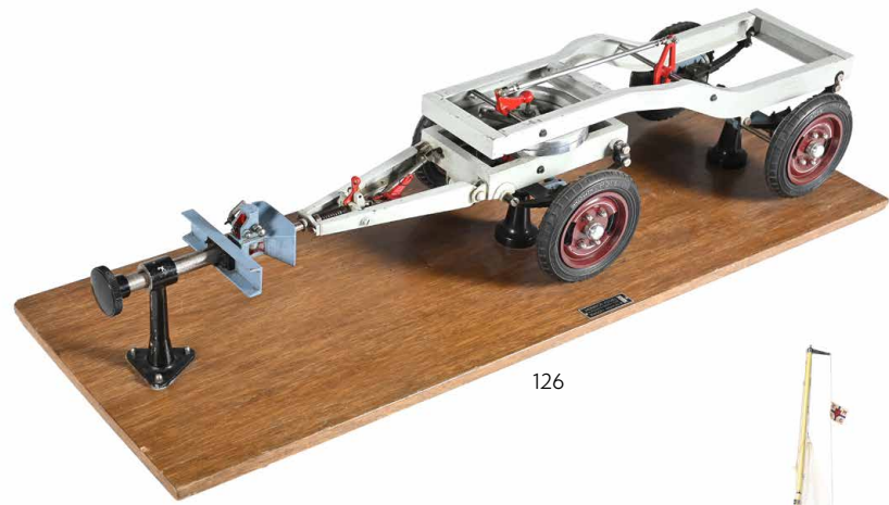
126 AN EXHIBITION MODEL OF A COMMERCIAL LORRY CHASSIS With detailed suspension and four-wheels with rubber tyres and articulated front axle. The model finished in grey paintwork with builders plaque ' Heninrich Vogel, Munchen 2, Kreuzstrafe 29. Serial number 36
