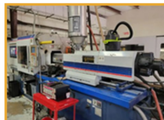
2001 Van Dorn 170HT720, Injection Molding Machine, Capacity 170 Ton, Shot Size 14.7 oz
