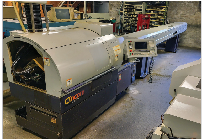
Citizen C16 16mm Swiss CNC Automatic Bar Machine
