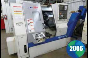
**DOOSAN-DAEWOO LYNX 220A CNC CHUCKING LATHE**
