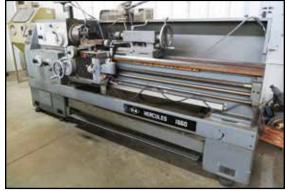
HERCULES 1660 16" X 60" ENGINE LATHE
