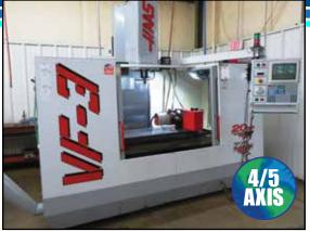
HAAS VF-3 4/5 AXIS CNC VERTICAL MACHINING **CENTER**
