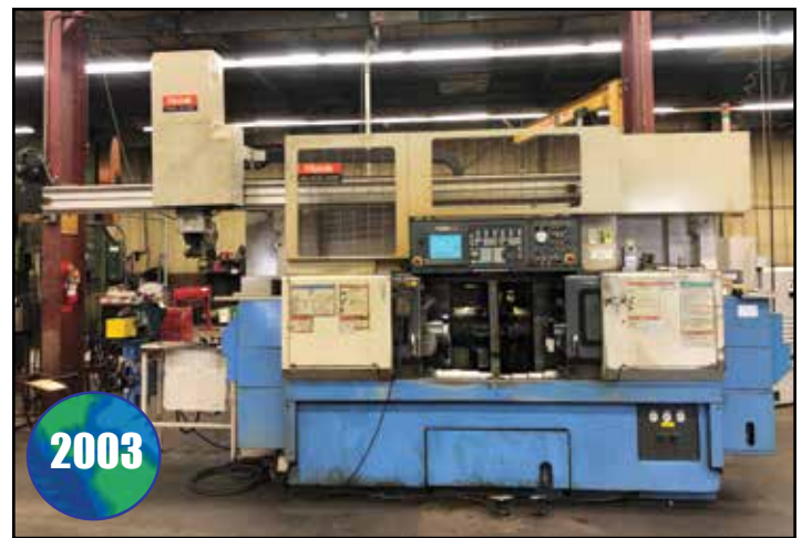
MAZAK MULTIPLEX 4200 DUAL SPINDLE CNC TURNING CENTER
