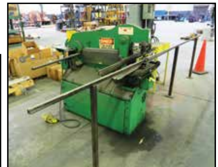
PIRANHA P3 50-TON HYDRAULIC IRONWORKER
