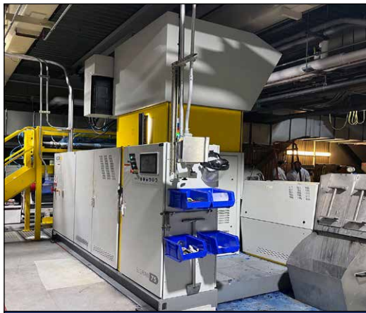
Views of NGR S: Gran 75 Plastics Shredder / Feeder / Extruder Combination Unit
