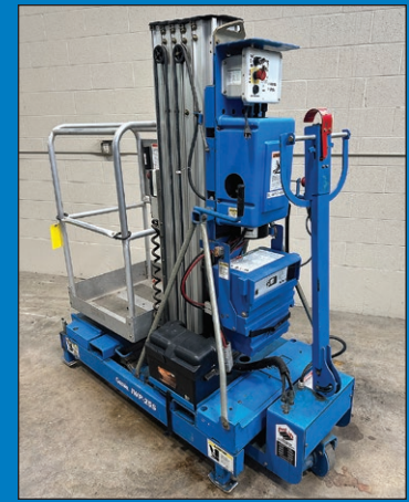
Genie Electric Manlift
