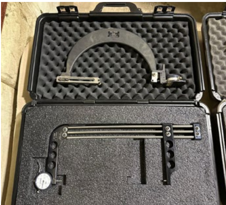
LOT OF 2: (1) GAGEMAKER EXTERNAL TAPER GAGE, (1) GAGEMAKER EXTERNAL THREAD ROLL GAUGE
