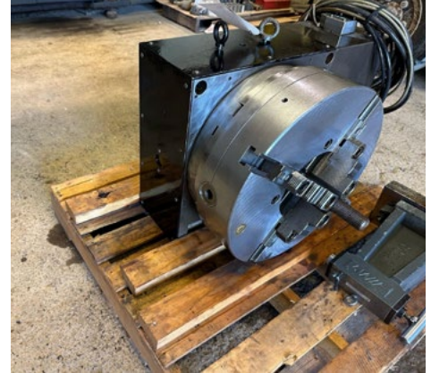
HAAS 4TH AXIS WITH 19" 4 JAW BISON CHUCK, MODEL HRT 450
