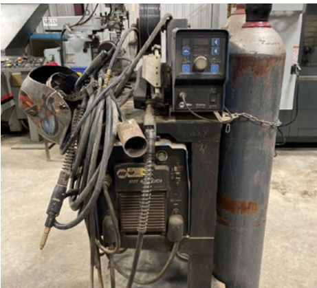
MILLER XMT 450 CC/CV WELDING POWER SOURCE ON CASTERS WITH MILLER 70 WIRE FEEDER
