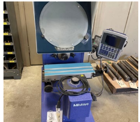
MITUTOYO PH-A14 HORIZONTAL PROFILE PROJECTOR WITH QM-DATA200 DATA PROCESSING UNIT
