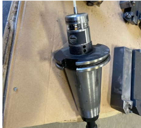
RENISHAW OPTICAL MACHINE PROBE 40-2 ON CAT 50
