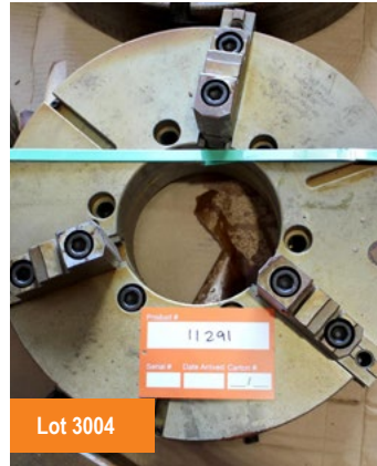
Lot 3004 19.5" 3-Jaw Chuck with 7.75" Thru-Hole
