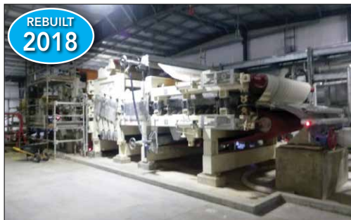
Hymac Wetlap Machine 100 HP-SF with Heavy Duty Press, Rebuilt 2018, (Rated 300-400 TPD)
