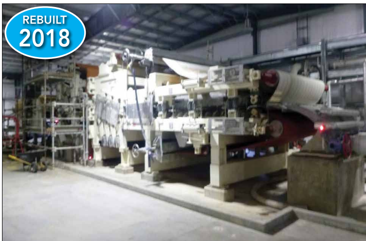
Hymac Wetlap Machine Model 100 HP-SF with Heavy Duty Press Rebuilt 2018 (Rated 300-400 TPD)
