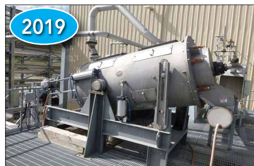
Vincent Model EF-30 Sludge Press S/S S/N 17590-8, Manufactured 2019
