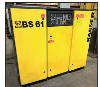
KAESER BS61 ROTARY SCREW TYPE AIR COMPRESSOR
