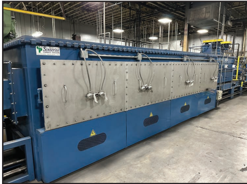
GASBARRE SINTERITE 24E-4Z-ADS-VERSACOOL RX BELT-TYPE FURNACE
