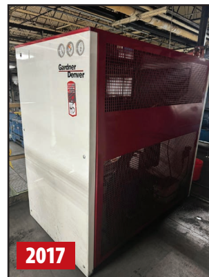
GARDNER DENVER GSRN-1200W-436 REFRIGERATED AIR DRYER
