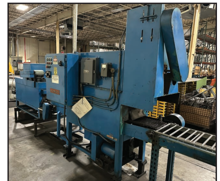
ALMCO RD12-48S BELT-TYPE PARTS DRYER
