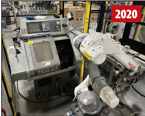
PO LY GIM MINI-88 CNC LATHE W/ NACHI ROBOT
