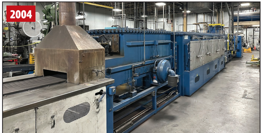
GASBARRE SINTERITE 24E-4Z-ADS-VERSACOOOL RX BELT-TYPE FURNACE
