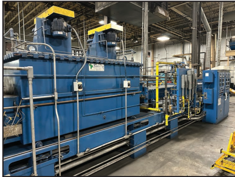
GASBARRE SINTERITE 24E-4Z-ADS-VERSACOOL RX BELT-TYPE FURNACE
