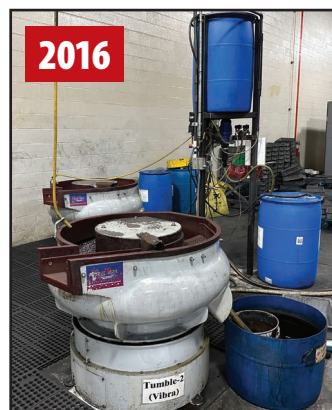
VIBRAHONE FCV 150 ULE-2 VIBRATORY POLISHING MACHINE
