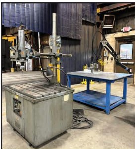
TAP DISINTEGRATOR & TAPPING ARM
