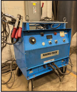
GOULD-BASS MAGNE-TECH MAGNETIC PARTICLE INSPECTION UNIT
