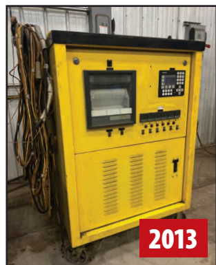
PDS BARTECH PRE/POST WELD INDUCTION HEATING SYSTEM
