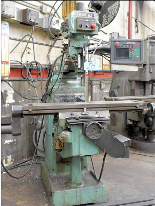
South Western Industries (SWI) Model TRAK-K3 EDGE, 3-HP Variable Speed CNC Vertical Milling Machine
