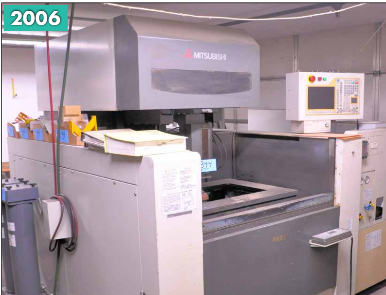
Mitsubishi FA20S CNC Wire Electrical Discharge Machine
