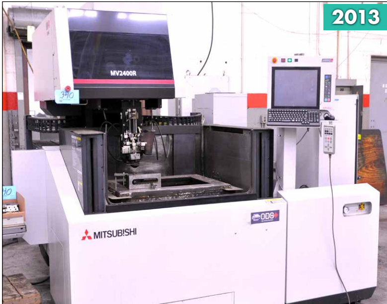
Mitsubishi MV-2400R Series Wire Electrical Discharge Machine
