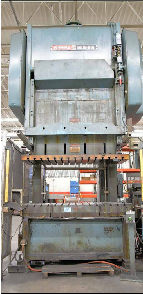
Niagra S2G-250-96-26, 250-Ton Capacity Air Clutch C-Frame Press
