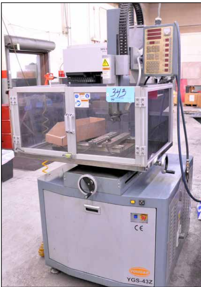
Yougar YG5-432 Small Hole Drilling Electrical Discharge Machine
