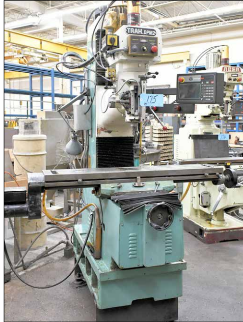
South Western Industries (SWI) Model TRAK-DPM EMX 2, 2-AXIS Variable Speed CNC Bed Milling Machine
