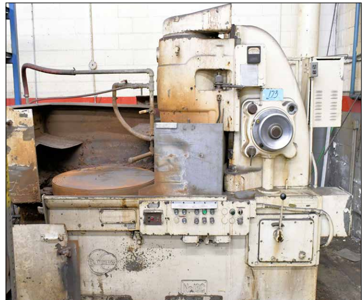
Blanchard NO. 18C Rotary Surface Grinder, 36" Diameter Magnetic Chuck
