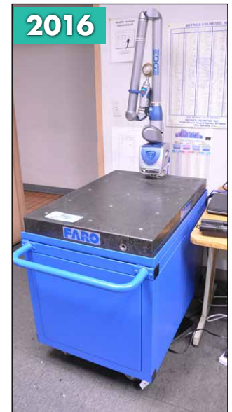
Faro Edge Coordinate Measuring Machine with Accessories
