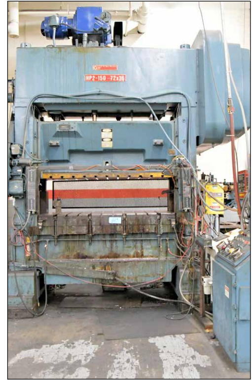
E. W. Bliss HP2-150 72x36, 150-Ton Capacity Air Clutch Straight Side Press
