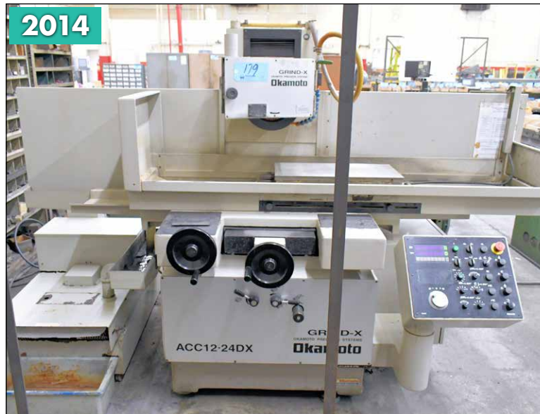
Okamoto Grind-X Model ACC 12-240DX, 12"x24" Hydraulic Automatic Surface Grinder
