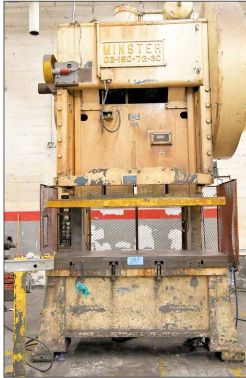
Minster G2-150-72-30, 150-Ton Capacity C-Frame Air Clutch Press
