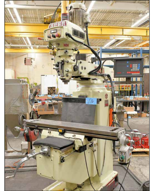
Acer E-Mill Model EVS-3VKH, 3-HP Variable Speed Vertical Milling Machine
