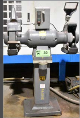
BALDOR 1406W 12" double end pedestal grinder
