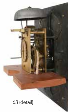
63 A GEORGE III THIRTY-HOUR LONGCASE CLOCK MOVEMENT AND DIAL PETER FEARNLEY, WIGAN, CIRCA 1775 The four-pillar countwheel bell striking two-handed movement with anchor escapement regulated by seconds pendulum and Huygens's endless rope winding, the 13 inch square brass dial with dummy winding squares, subsidiary seconds dial and shaped silvered plaque signed FEARNLEY, WIGAN to the unusual diamond lozenge hatched matted centre, within applied Roman numeral chapter ring with calendar scale to inside track and Arabic five minutes beyond the dot minute track, with scroll pierced steel hands and applied gilt brass rococo scroll cast spandrels to angles, (calendar work incomplete); now with an oak wall bracket and simple box hood cover of recent construction. The movement 33cm (13ins) square, 15cm (6ins) deep including crutch.
