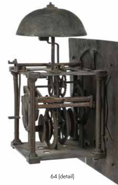
64 A QUEEN ANNE POSTED THIRTY-HOUR LONGCASE CLOCK MOVEMENT WITH TEN-INCH DIAL UNSIGNED, PROBABLY LANCASHIRE, EARLY 18th CENTURY The countwheel bell-striking movement with separately wound trains, anchor escapement for regulation by seconds pendulum and well detailed column-turned corner posts, the 10 inch square brass dial engraved with stylised urn and tulip blooms within applied Roman numeral chapter ring with large sword-hilt half hour markers, with scroll-pierced brass hand and cast figural spandrels emblematic of the four seasons to angles, (no pendulum or weights). 33cm (13ins) high, 18cm (7ins) deep overall.
