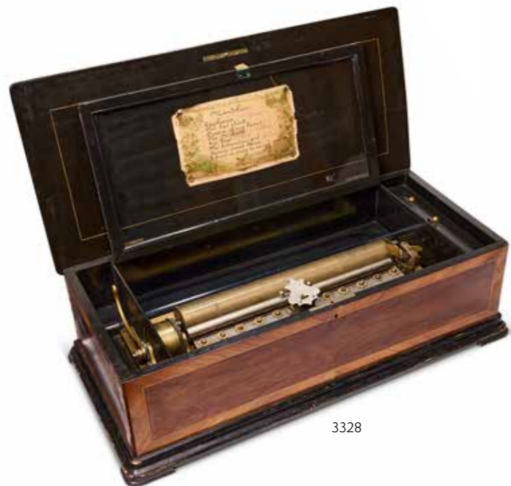
328 Y A SWISS ROSEWOOD AND INLAID MUSICAL BOX LATE 19TH CENTURY, RETAILED BY IMHOF & MUKLE Playing a choice of eight airs via a pinned brass cylinder and tuned steel combs, the movement driven by a single wound spring drum mounted on a gilt iron bed beneath a hinged glass internal cover, marked for the retailer, and with selection levers to the side, the lid with applied printed and hand written tune sheet serial numbered 39967, the case of typical rectangular form with marquetrie inlaid lid 24cm high, 78cm wide, 36cm deep
