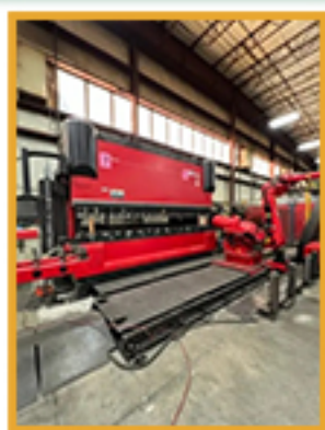
2011 Amada HDS 2204NT, 243 Ton x 14' Hydraulic Press Brake w/ Astro 165W NT Robotic Bending System
