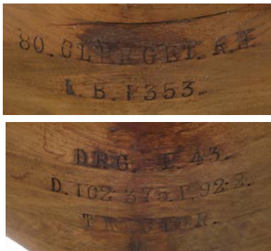
369* Propeller. French walnut two-blade propeller, early 20th century, the boss stamped 80 CLERGET R.H. I.B. 1353, the opposite side stamped DRG P.43, D.102 375. P.922, TRACTOR, approximately 261 cm
