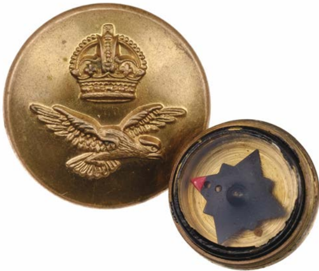
347* Escape Compass. WWII RAF/SOE button compass by Gaunt & Son, London, unscrews to reveal a small airman's rotor compass, 23 mm diameter (1)
