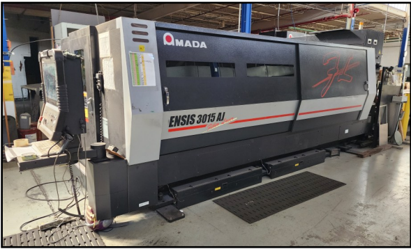
2016 Amada Ensis 3015AJ Fiber Laser w/Shuttle Table, Scissor Lift Table, Safety Light Curtains, Chiller & Dust Collector
