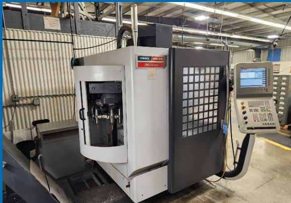
DMG Mori Model DMU50 ECO CNC Five Axis Universal VMC (2011)
