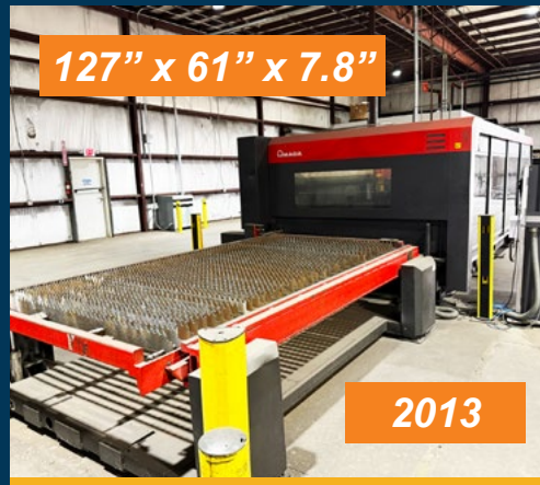
AMADA 4000 WATT CO2 LASER CUTTING MACHINE
