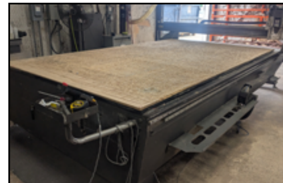
MULTICAM 3000 SERIES CNC ROUTER S/N 3-305-R-FP071 (1996) 84" X 148" TABLE, PENDANT CONTROL, VACUUM SYSTEM
