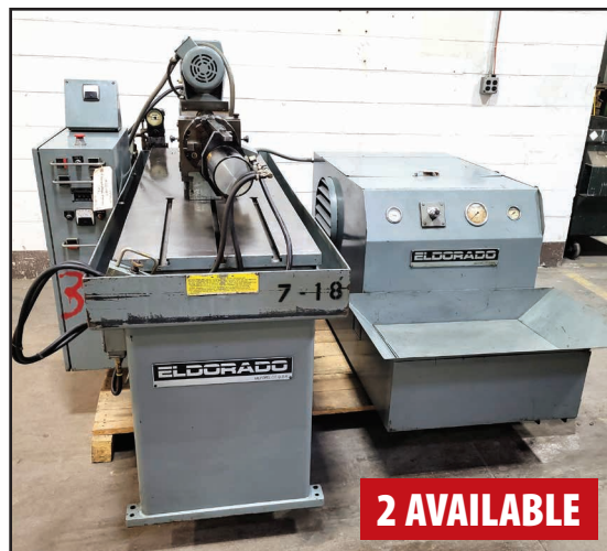
ELDORADO MEGA M-75-1041 3/4" X 30" PRECISION DEEP HOLE GUN DRILL
