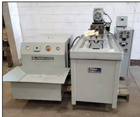
ELDORADO MEGA M-75-1003 3/4" X 15" PRECISION DEEP HOLE GUN DRILL
