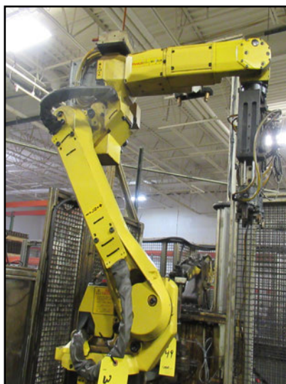
Fanuc M-10iA 6-Axis Robot w/R-30iA Controller & Dual Schunk 3-Jaw Grippers on Air Slides
