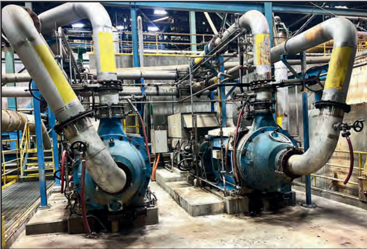
(2) METSO CONFLO CONICAL REFINERS WITH WITH 2,100 HP DRIVE
