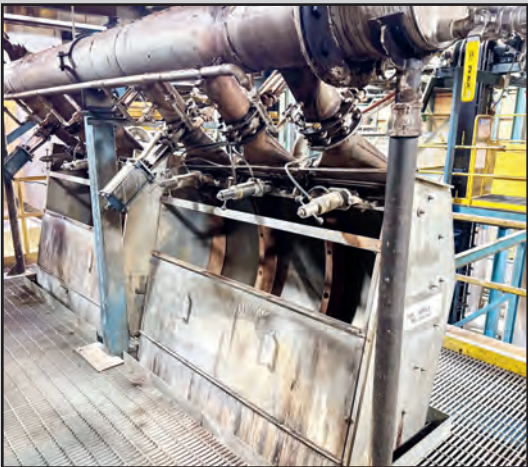
316 SS 12" DIA. AUGER CONVEYORS
