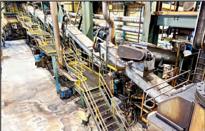
316 SS 12" DIA. AUGER CONVEYORS
