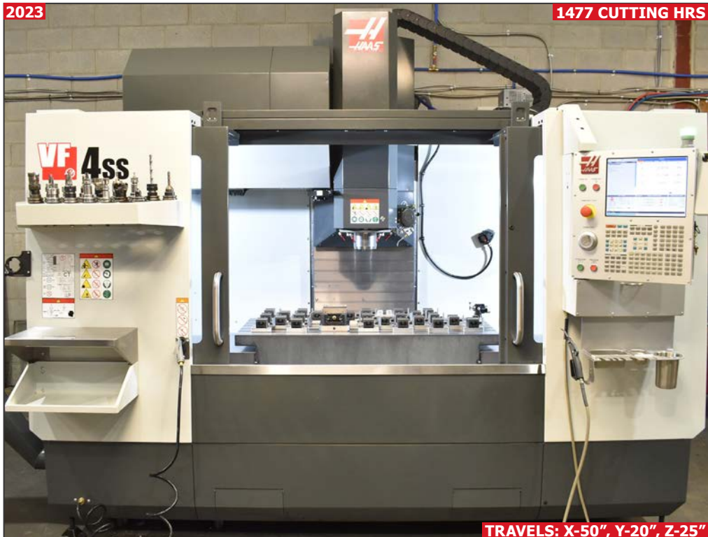
HAAS VF-4SS CNC high speed vertical machining center
