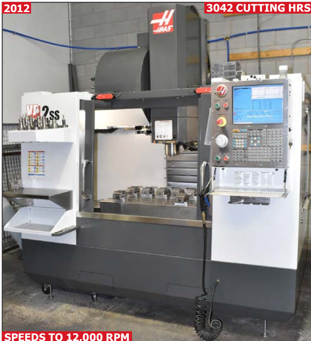
HAAS VF-2SS CNC high speed vertical machining center
