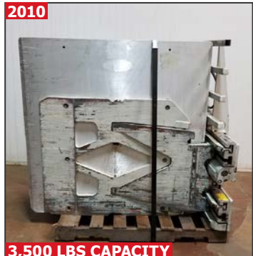
CASCADE RU35D-CCS-35Q hydraulic rotary carton clamp forklift attachment
