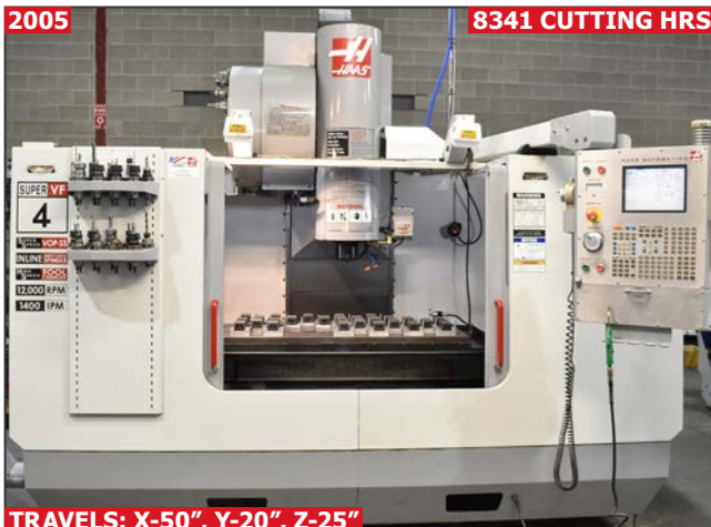
HAAS VF-4SS 5-axis ready CNC high speed vertical machining center
