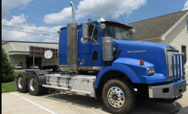
2012 Western Star 4900SA Cummins ISX 485hp, Jake, Allison 45000RDS, Air Susp, 13/40k Axles, 4.11 Ratio, Quadlock, 26k mi
