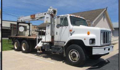
2001 International 2574 Cat C10 305hp, Retarder, Allison HD4560, Air Susp, 214" WB, 16/46k Axles, Altec 30k Boom, 11k mi
