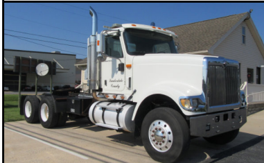
2006 International 5900i Cummins ISX 475hp, Jake, 10 Spd, Air Ride, 13/46k Axles, 3.73 Ratio, 218" WB, ¾ Locks, 111k mi
