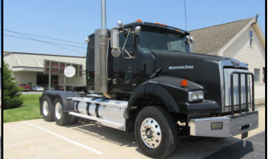
2012 Western Star 4900SA 34" Sleeper Det DD13 450hp, Jake, 10 Spd, Air Susp, 12/40k Axles, 3.90 Ratio, Quadlock, 210" WB, 27k mi
