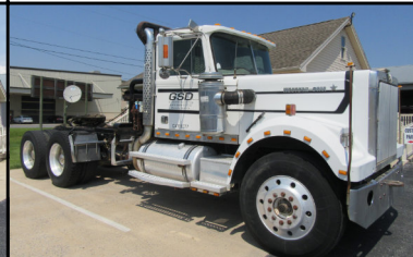
1985 Western Star 4964 Cummins NTC 400hp, 13 Spd, Spring Susp, 12/38k Axles, 217" WB, 2 spd aux. Trans, 279k mi
