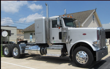
2015 Peterbilt 389 36" Sleeper Cummins ISX15 485hp, Jake, 18 Spd, Air Susp, 14/46 Axles, 3.91 Ratio, Quadlock, 32k mi
