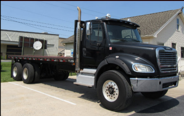
2013 Freightliner M2 Flatbed Cum ISL 380hp, Exh. Brake, 10 Spd, TuffTrac Susp, 20/46k Axles, 189" CT, Dble Frame, 22' Bed, 223k mi
