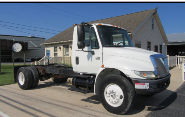
2007 International 4300 DT466E 245hp, 6 Spd, Spring Susp, 12/21k Axles, 4.11 Ratio, 129" CA, 13' of Frame, 42k mi
