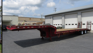
2016 Kauffman Equip. Trailer 43' x 102" Spring Susp, 55k GVW, Ramps for upper deck
