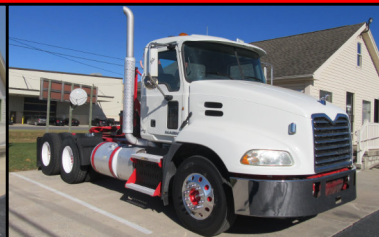
2011 Mack CXU613 MP8 415hp, Jake, 10 Spd, Air Susp, 12/40k Axles, 3.90 Ratio, 187" WB, Quadlock, Wetline, 35k mi
