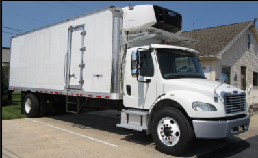
2019 Freightliner M2 Cummins B6.7 280hp, Exh Brake, Allison 2500RDS, Air Susp, 33k GVW, 285" WB, 26' Box, Good Reefer, 211k mi
