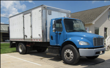
2017 Freightliner M2 Cummins ISB 240hp, Exhaust Brake, Allison 2500RDS, Air Susp, 33k GVW, 204" WB, 18' x 102" Box, 180k mi
