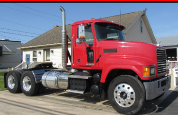
2012 Mack CHU613 MP8 415hp, Jake, 13 spd, Camelback Susp, 14/44k Axles, 4.19 Ratio, 207" WB, 42k mi
