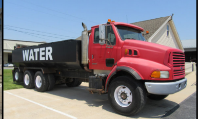
1999 Sterling LT9500 Tanker Cat 3406 435hp, Jake, 8LL, Hend. Susp, 18/40k Axles, 4.11 Ratio, Quadlock, 21' Tank, 169k mi
