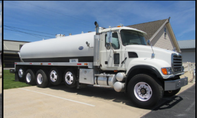
2007 Mack CV713 Tanker Mack AI 427hp, Jake, 10 Spd, Hend Susp, 20/46k Axles, 275" WB, Quadlock, 4750 gal. Tank, 153k mi
