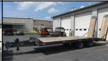
1989 Eager Beaver Pintle 23' x 96", 17' Deck w/5' Tail, 9' Ramps, Spring Susp, 25k GVW
