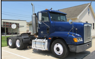
1999 Freightliner FLD120 Detroit 12.7L 430hp, Jake, 10 Spd, Air Susp, 12/40k Axles, 3.9 Ratio, 178" WB, 132k mi
