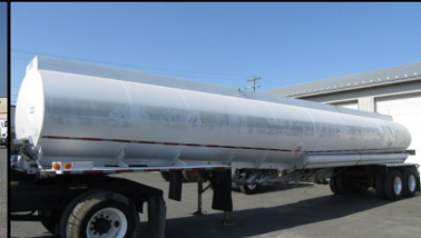
1985 Heil Aluminum Tank Trailer 9000 Gal, 43' x 96", Spring Susp
