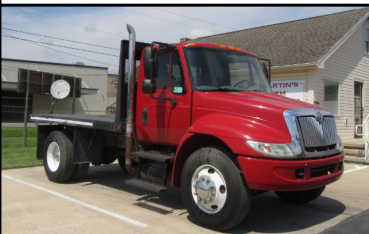
2003 International 4300 Flatbed DT466E 250hp, 10 Spd, Spring Susp, 10/23k Axles, 165" WB, 139k mi
