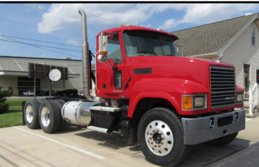
2011 Mack CHU613 MP8 415hp, 13 Spd, Camelback Susp, 14/44k Axles, 4.19 Ratio, 207" WB, 100k mi
