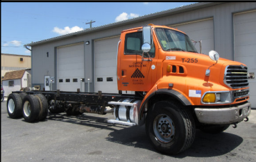
2007 Sterling LT9500 (Non Runner) Mercedes MBE 4000 410hp, Jake, Allison 4500RDS, TuffTrac Susp, 20/46k Axles, Quadlock, 150k mi
