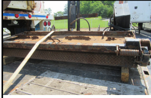
Maxon Tuk-a-way lift gate 2,500 lb. capacity
