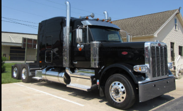
2024 Peterbilt 589 80" Sleeper Cummins X15 500hp, Jake, 13 Spd, Low Low Air Leaf Susp, 13/40k Axles, 3.25 Ratio, 280" WB, 113k mi
