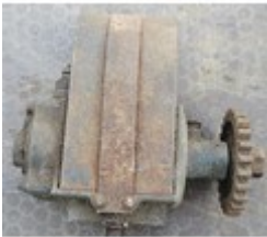
117. A stationary engine low tension magneto
