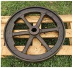
25. A Lister stationary engine flywheel
