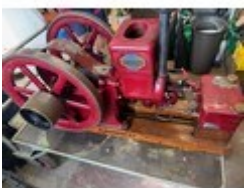
268. An AMANCO Waterloo 2 1/2hp stationary engine, hopper cooled "Hired Hand", serial number 137352
