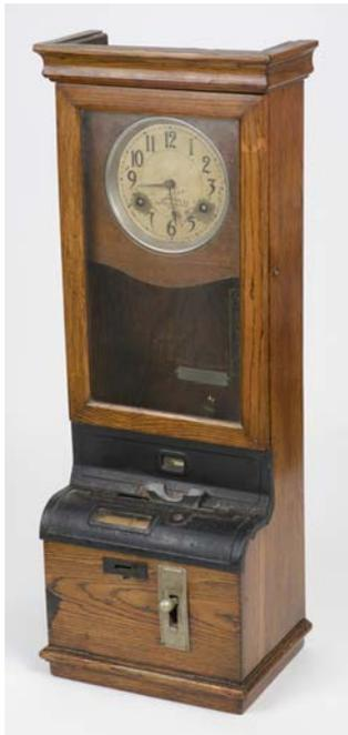
742\* **Time Recorder.** International Time Recording Co Ltd London "clocking in machine", circa 1920, oak case with stores reference plate stamped 'Model No 950, Serial No 351381, Ink Ribbon 11', 101 cm high
