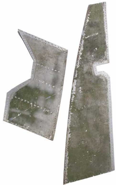
488* Supermarine Spitfire. Two Mk 16 Spitfire aileron skins from TD248, aluminium sheet metal with rivet holes to the edges, finished in green, 135 cm and 65.5 cm long
