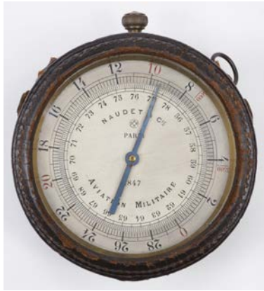
397* Aviation Altimeter. A WWI French aircraft altimeter by Naudet & Cie, Paris, the 70 mm circular silvered dial with blued steel hand, signed 'Naudet & Cie Paris, 2487 Aviation Militaire, numbered 56-78 inclusive, with a revolving brass chapter dial numbered 0 - 28 inclusive, the brass case with a large winding crown, case size approx. 100 mm, with brown leather case (1) £300 - £500
