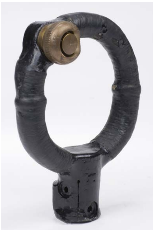
481* Spade Grip. WWII Mk 1 Spitfire spade grip, black painted finish with rubberised grip, the frame stamped 'AH 2040' with brass pneumatic gun button stamped 'Safe' and 'Fire', the opposite side stamped 'M2', 19 cm long
