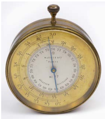
398* Aviation Altimeter. A WWI French aircraft altimeter by Naudet & Cie, Paris, the 55 mm circular silvered dial with black steel hand, signed 'Naudet & Cie Paris, No 27 Aviation Militaire, numbered 56-76 inclusive, with a revolving brass chapter dial numbered 2 - 50 meters inclusive and, the brass case with a large winding crown, case size 100 mm (1) £200 - £300
