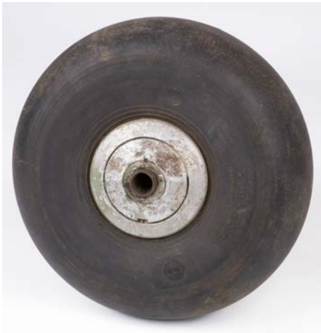
490* Tail Wheel. WWII RAF Spitfire/Hurricane tail wheel, with aluminium hub and rubber tyre numbered 495- 3 1/2, Electrically Conducting, various other markings, approximately 30 cm diameter
